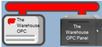
Figure 15 - Enabled OPC Driver that is not communicating with the Driver Service
