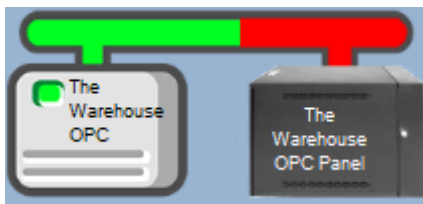
Figure 16 - Enabled OPC Driver that is communicating with the Driver Service but NOT the panel
