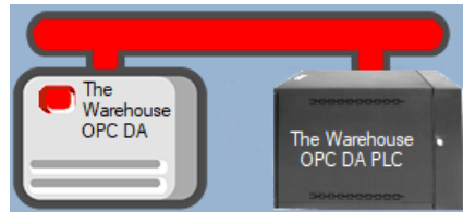
Figure 18 - Enabled OPC DA PLC Driver that is not communicating with the Driver Service
