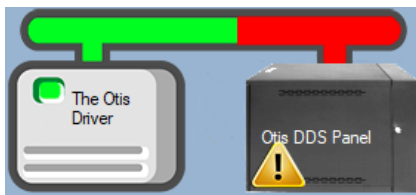
Figure 21 - Enabled Otis Driver that is communicating with the Driver Service but NOT the panels
