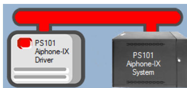
Figure 18 - Enabled Aiphone-IX Driver that is not communicating
