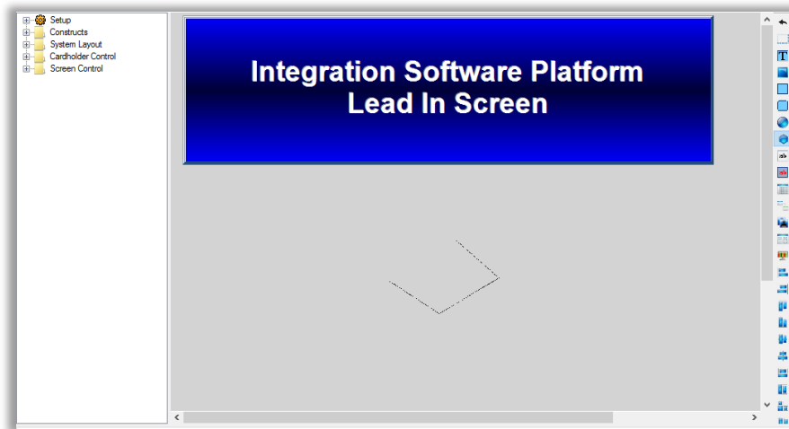
Figure 57 - A polygon screen object while being drawn
