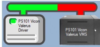
Figure 13 - Enabled Vicon Valerus Driver that is communicating with the Driver Service but NOT the panel
