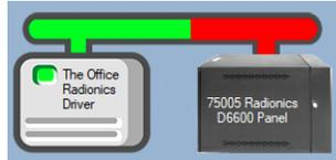
Figure 17 - Enabled Radionics Driver that is communicating with the Driver Service but NOT the panel
